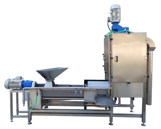
During washing, the surface of the grain is cleaned, any heavy or ligh dirt and shrunk seeds are separated out, and microorganism are removed.
