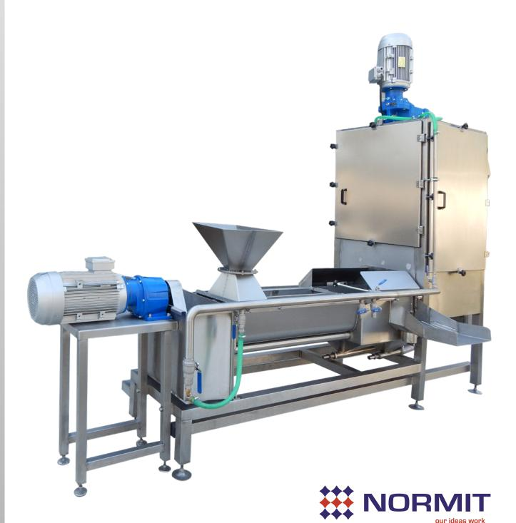
Wetting and washing grain is a process done to prepare it for milling. When wetting is carried out, psysicbiological processes take place in the grain, and as a result, it becomes easier to separate the husk from the grain with minimal losses of the grain endosperm.
