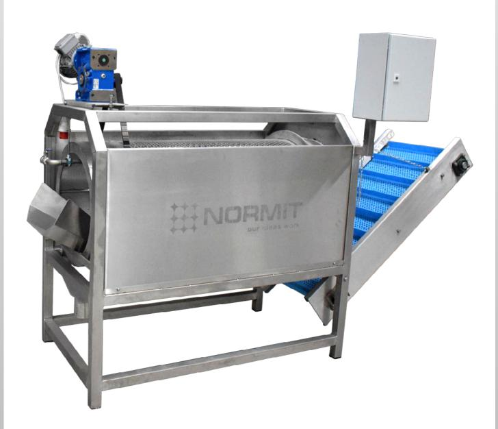
Washer is an effective solution for washing potatoes, carrots, beets, and other root vegetables, including highly dirty ones with a large amount of soil, clay and other impurities stuck to them. The process of vegetable cleaning is carried out through friction between the product and the perforated walls of the drum, or between the vegetables themselves, and also through water rinsing.
